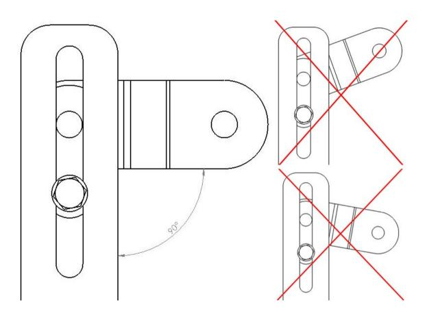
ATTENTION: The exact setting of mounting height is not only a prerequisite for accurate weighings. When the angle is not exactly right, the three-point scale and/or your implement could get damaged or deformed.
